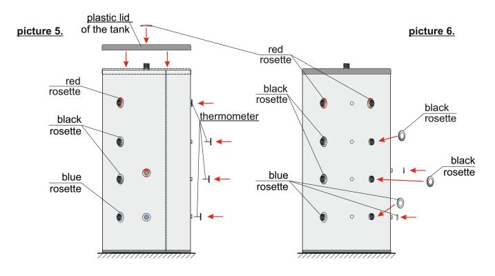
On the connections placed the rosette and on the plastic lid glue the stickers on the opening for the connections (picture 6. and picture 7.)
