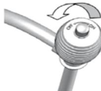
Finish filling the stove tank, turn the knob off, turn it anticlockwise. This way you empty the siphon pump
